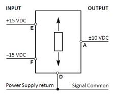
A through F: Connector pin assignments
