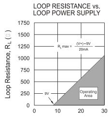
Loop Power Supply Voltage,  $V_{PS}(V)$
