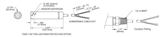
**Gland Cable Seal Configuration for ETFE Cable**
