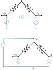
Constant Current Mode: Current level should be chosen for patient safety, signal-tonoise and lifetime requirements. (Blue portions of circuit supplied by customer.) Refer to ISO 60601 for patient risk current safety limits.
