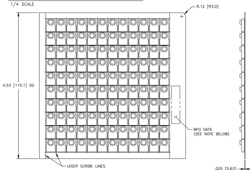
NOTE: MFG DATA CONSISTS OF LOT NUMBER, MODEL NUMBER AND QUANTITY OF GOOD UNITS PER SUBSTRATE PANEL.
